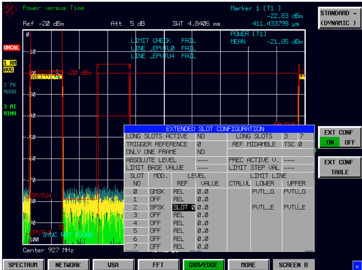
Fig. 2-8 Dynamic extended slot configuration – incorrect level profile>
