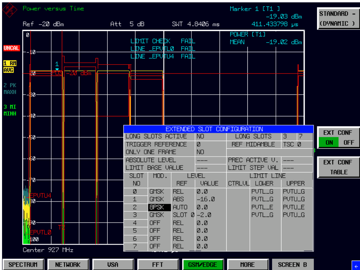
Fig. 2-9 Dynamic extended slot configuration – incorrect level
